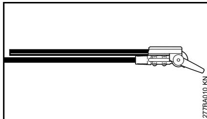
For compact transport of the machine, in this version, the cutter bar can be swung parallel to the shaft and locked in this position.
