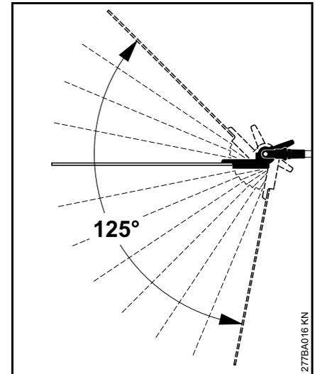
In this version, the angle of the cutting bar relative to the shaft is adjustable from 0° (completely straight) to 45° (in 4 stages upward) and to 80° (in 7 stages downward). Twelve individually adjustable working positions are possible.
